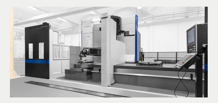
The machine is also equipped with the new SORALUCE H200T multifunction head for turning and milling operations. The H200T head is equipped with an innovative spindle rotation locking system, allowing the use of both milling and turning tools directly without the need for intermediate elements.
