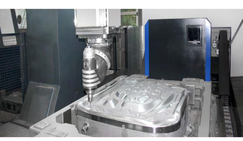
"Each moulding tool requires an average of 5 days of polishing at Audi before it can be installed in the press. I'm impressed by the precision of the new portal milling machine from Soraluce. It's so accurate, even on radio profiles, that we only need 3 days for polishing".
